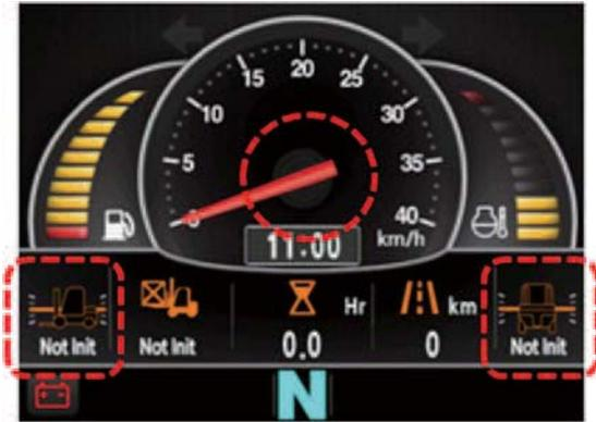
2) Vehicle that has applied the mast angle sensor
